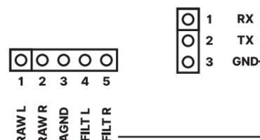
**J12: UART.** Connect a USB-to-UART cable to RX, TX and GND pins (115200 baud) to see ZZ9000's debug output.
