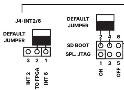
**J4: Interrupt select.** Connects either Amiga interrupt INT2 or INT6 to the FPGA. Leave the jumper on INT6 to use Ethernet.
