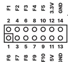
**J10: FPGA Expansion.** 10 additional unused FPGA inputs/outputs for later use.
