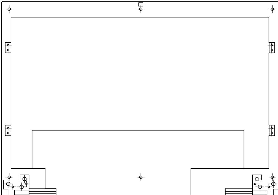
The display is mounted on the screen back with M2x4 screws. The left and right hinges are mounted in the bottom left and right corners with M4x5 screws.
