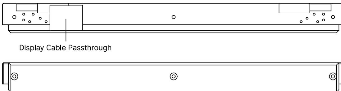
The screen support connects the main box to the screen via the hinges. The display's LVDS (motherboard header J14) and power cable (motherboard header J26) is passed through this part, as well as the lid sensor cable (J34).
