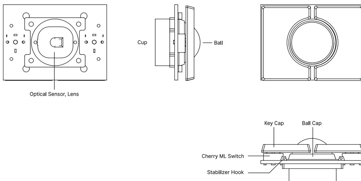
The trackball uses the same microcontroller and LUFA framework as the keyboard, but instead of scanning a matrix of switches, it gets X and Y movement coordinates from the PMW3360DM-T2QU optical sensor that is connected via SPI.
