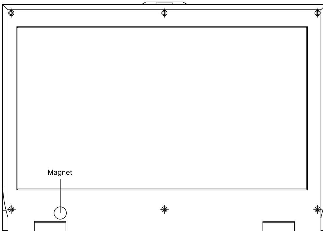
This part serves as a bezel for the display and holds the case closing strap. It also has a magnet attached to it on the lower left that is sensed by the lid sensor. The screen front is mounted to the back with M3x6 screws.
