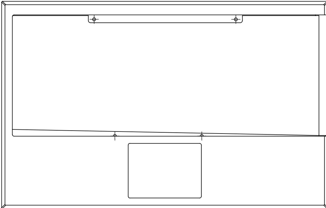
The main box top is pressed onto the main box to close it from the top. It acts as a palm rest and bezel for the keyboard and trackball. The keyboard is slid into this part's keyboard slot from the right.
