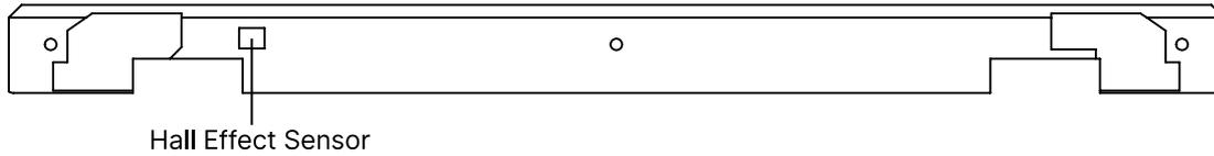
This is a thin part covering the screen support's top. On the left, it contains a pocket for the hall effect sensor that detects the magnet on the screen front. The sensor signals opening and closing of the lid.
